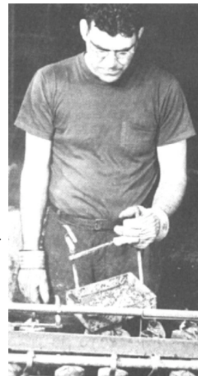
CADMIUM PLATING Slugs are placed in baskets for cadmium plating, which provides additional hardening
