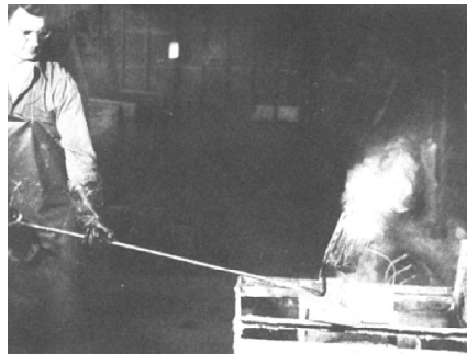
HARDENING BATH —newly pressed slugs are bathed in cyanide at 1600°.
