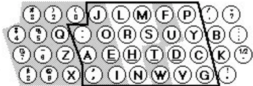
RIGHT: Keyboard designed by August Dvorak for typing with the right hand alone. Most typing done on keys within black border. TOP RIGHT: One-armed veteran of World War One types on a Remington 10.
